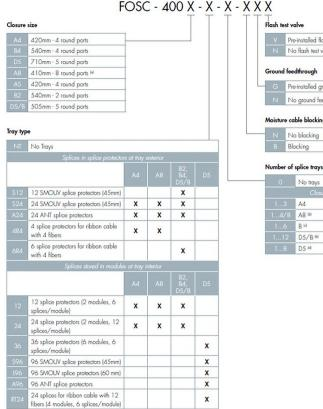
Flash test valve V Pre-installed flash test valve No flash test valve Ground feedthrough © Pre-installed ground feedthrough N No ground feedthrough
