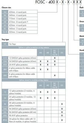
Flash test valve Pre-installed flash test valve No flash test valve Ground feedthrough © Pre-installed ground feedthrough N No ground feedthrough
