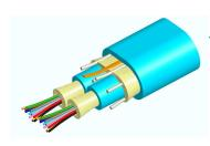
Fiber indoor cable, LazrSPEED®, Low Smoke Zero Halogen Riser MPO Trunk, 24 fibers, 12 fiber subunits, Multimode OM3, Gel-free, Feet jacket marking, Aqua jacket color, B2ca flame rating
