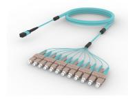
OM3 MPO (Unpinned) to SC/UPC, InstaPATCH  $^{\odot}$  360 Array Cord, 12-Fiber, Plenum
