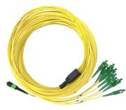
Multi Distribution Break Out Cable Singlemode MPO/8 equipment unpinned to SC/APC, 8 fibers, LSZH, 8 meters
