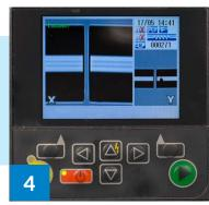
The display shows the quality of the fusion splice Spliced fibers and protective sleeve (SMOUV)
