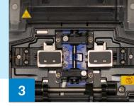
Fibers are joined in a fusion splicer
