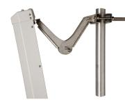
Downtilt Mounting Kit for 2.4 - 4.5 in (60 - 114 mm) OD round members. Kit contains one scissor top bracket set and one bottom bracket set.
