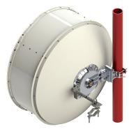
1.2 m | 4 ft Sentinel® High Performance Antenna, dual-polarized, 5.925–7.125 GHz, PDR70, white antenna, flexible woven polymer gray radome without flash, standard pack—one-piece reflector
