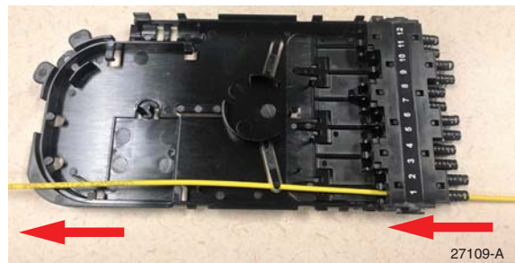
Figure 2. Pulling cable through cassette
