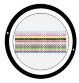
CommScope's rollable ribbon technology utilizes partially bonded fiber ribbons comprised of 12 fibers. Unlike conventional ribbons, which are fully longitudinally bonded, rollable ribbons are partially bonded. As seen below, the partial bonding process used with rollable ribbons allows them to be easily separated and "rolled" into a cylinder, thus making much better use of space when compared with flat ribbons.
