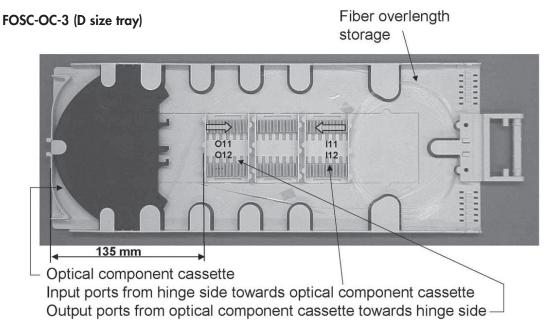
5.1 The above drawing shows the dedicated spaces (in the D tray) where the fibers are to be stored after splicing
