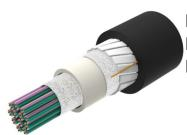
Fiber OSP cable, Non-Armored, All-Dielectric, Arid-Core, Dry Central Tube Rollable Ribbon, 288 fiber, Singlemode G.652.D and G.657.A1, Gel-free, Feet jacket marking, Black jacket color
