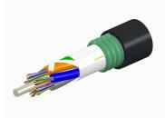
Fiber OSP cable, LightScope ZWP® Single Jacket/Single Armor, 84 fiber, Gel-Free, Stranded Loose Tube, Singlemode G.652.D and G.657.A1, Meters jacket marking, Black jacket color
