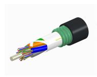
Fiber OSP cable, LightScope ZWP® Single Jacket/Single Armor, 64 fiber, Gel-Free, Stranded Loose Tube, Singlemode G.652.D and G.657.A1, Meters jacket marking, Black jacket color
