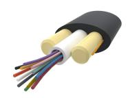
Fiber outdoor drop cable, LightScope ZWP® Self-Supporting All-Dielectric, Singlemode G.652.D and G.657.Al, 4 fiber Arid Core construction, Gel-filled, central loose tube, Meter jacket marking, Black jacket color
