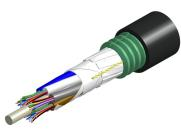
Fiber OSP cable, LightScope® ZWP Mini Single Jacket/Single Armor, 12 fiber, Gel-Filled, Stranded Loose Tube, Singlemode G.652.D and G.657.Al, Meters jacket marking, Black jacket color
