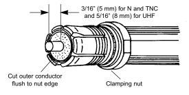
**5** Separate Foam from Outer Conductor. Insert the tip of a knife to a depth of 1/16 inch (1.6 mm) between the foam and the outer conductor of the cable and separate them so that the outer conductor can be flared. Move the knife around the entire circumference of the outer conductor. Scrape away any foam clinging to the outer conductor and remove any burrs from the inside edge. Remove copper particles from the foam with a wire brush.
