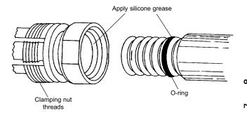
Add Clamping Nut and Cut Cable. Push the clamping nut fully onto the cable with a twisting motion so that the spring contacts snap into the conductor groove and the O-ring seats properly against the inside surface of the clamping nut. Check that the conductor cut line is aligned with the edge of the clamping nut.
