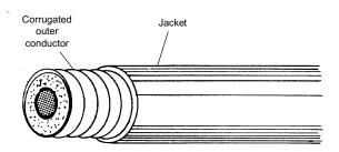
Mark Conductor and Remove Jacket. Scribe a cutting line with a knife on the ridge of exposed, corrugated outer conductor. Remove the jacket to the dimension shown, using a straight-edged piece of heavy paper wrapped around the cable to guide the cut.
