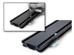
Assemble screw and washer in the T-channel Use an Allan key n°5 with conical head Bracket needs to be fixed with a torque of 3.5-4Nm
