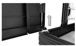
Pull the pin on the bottom side of the door up Align the pin with the hole in the hinge bracket Release it and check if the pin is fixed in the hole The door is fixed in the frame now
