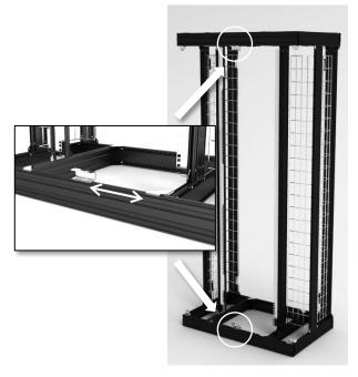
Assemble both hinge brackets with screws and washers in the middle of the horizontal profiles on the front side of the frame See 2.2. how to fix the hinge bracket in place Check the positions of the brackets by measuring the distance of 176mm from bracket to bracket
