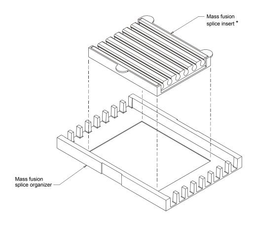
\* When using the mass fusion splice organizer assembly for silicon optical bench (SiOB) coupling, the couplings can be stored in the splice organizer with or without the splice insert.
