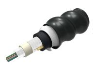
Fiber Indoor/outdoor Cable, Interlocking Armored, Low Smoke Zero Halogen (LSZH), Riser-Rated, 96 fiber, Gel-Free, Central Tube Ribbon, Singlemode G.652.D and G.657.A1, Feet jacket marking, Black jacket color
