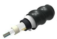
Fiber Indoor/outdoor Cable, Interlocking Armored, Low Smoke Zero Halogen (LSZH), Riser-Rated, 96 fiber, Gel-Free, Central Tube Ribbon, Singlemode G.652.D and G.657.A1, Feet jacket marking, Black jacket color
