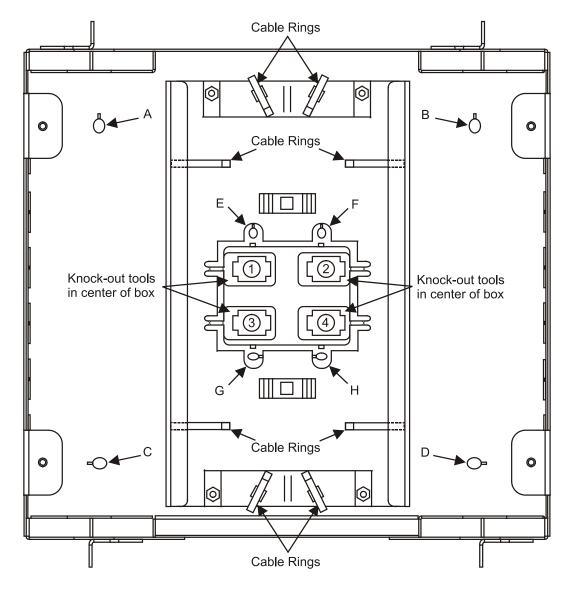
Figure 2 — Mounting Hole Locations
