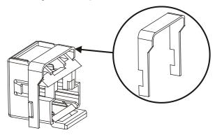
Figure 4 — Retention Clip Shown on Module
