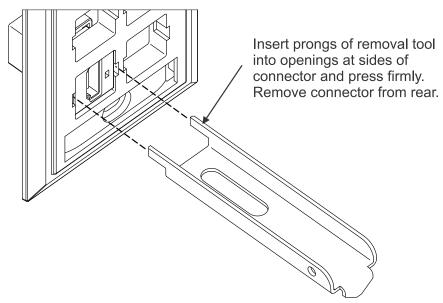
To remove a connector for inspection or repair, insert prongs of removal tool into openings at sides of connector and press firmly. Remove the connector from the rear.
