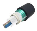
Fiber OSP cable, Steel Armored, Arid-Core, Dry Central Tube Ribbon, 72 fiber, Singlemode G.652.D and G.657.A1, Feet jacket marking, Black jacket color
