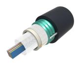
Fiber OSP cable, Steel Armored, Arid-Core, Dry Central Tube Ribbon, 288 fiber, Singlemode G.652.D and G.657.A1, Feet jacket marking, Black jacket color
