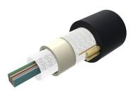
Fiber OSP Cable, Non-Armored, All-Dielectric, 576 fiber, Arid-Core, Dry Central Tube Ribbon, Singlemode G.652.D and G.657.Al, Gel-free, Feet jacket marking, Black jacket color
