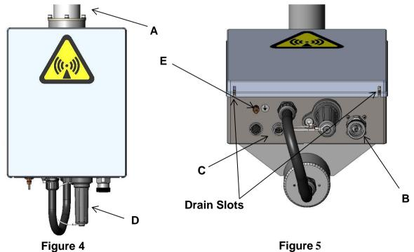
Figures 4 & 5 above show Normal Control Box Orientation. (Looking from front & bottom)
