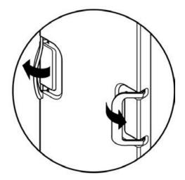
Detail B - Open Both Handles To Remove Door
