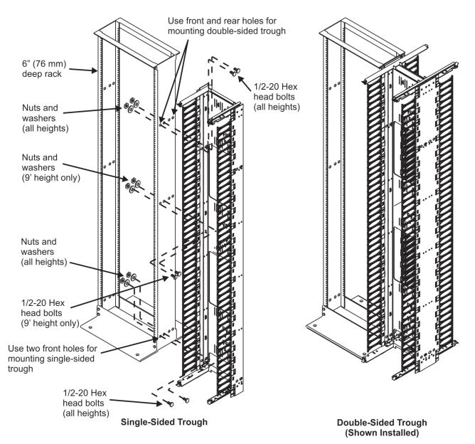
**Note:** Single-sided and double-sided vertical cable management kits are mounted to a rack using the provided 1/2-20 hex head bolts, washers, and nuts. The 7-foot (2.1m) and 8-foot (2.4m) heights use four bolts, washers, and nuts, whereas the 9-foot (2.7m) height uses six bolts, washers, and nuts as shown in the figure above.
