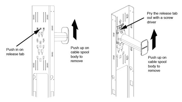
7. The spool (MID:860402049) is also applicable, could be ordered as a spare kit. Install it into vertical cable management trough by placing tabs, on rear of spool, into openings provided in back of the vertical cable management trough. Push down on spool until it snaps into place. To remove it, extend one hand through the opening in rear of cable manager closest to the spool and push in on release tab on lower part of the spool as shown. At the same time, push upward on body of cable spool.
