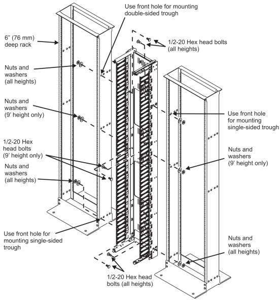
Single-Sided Trough Installed Between Two Racks
