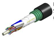
Fiber indoor/outdoor cable, loose tube gel-filled CST, 72 fiber, Singlemode G.652.D and G.657.A1, Meters jacket marking, Black jacket color
