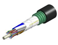
Fiber indoor/outdoor cable, loose tube gel-filled CST, 72 fiber, Multimode OM3, Meters jacket marking, Black jacket color
