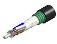
Fiber indoor/outdoor cable, loose tube gel-filled CST, 72 fiber, Multimode OM4, Meters jacket marking, Black jacket color
