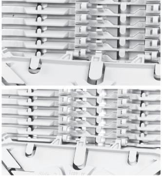
4.4 Place a tray in the wraparound groove plate; do this by pushing the lip on the groove plate (lowest possible position) slightly down with the tray and move the tray lateral into the hinge-cavities of the groove plate. To snap the High Capacity Single Element tray (HCSE) in the W/a single fiber groove plate leave always one hinge facility open between Fasblock or previous tray and the HCSE-tray.
