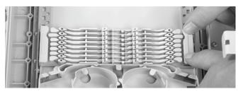
4.2 To remove push the two snapfits at S2 UMS-profile and slide the wraparound plate towards S1 UMS-profile.
