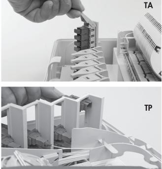
6.1 Slide the patch panel upwards up till the first locking position, not further.
