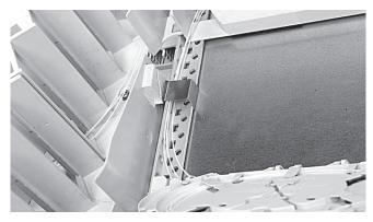
4.3 If box is not completely filled with groove plates, use pigtail clip retainer to hold the pigtails in place in the open area.
