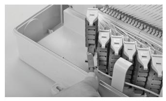
7.1 Slide the patch panel upwards until the first locking position, not futher. Connect the pigtail/patch cord into the designated adaptor.
