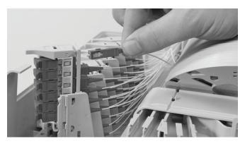
6.3 Route the pigtails towards the tube holder, different grooves can be used to separate the bundle of pigtails if needed.
