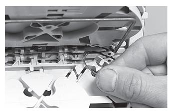
4.6 Position the wedge carefully such that the groove is still accessible for the fibers and be careful not to push the wedge against fibers. To remove the wedge, use two hands to pull on both ends (near the groove plate). Route the fiber in the grooves of the wraparound groove plates to the entrance of the identified tray. Fiber must be routed in the groove below the hinge of the tray!
