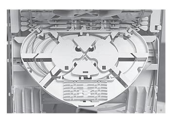
4.8 Store the fibers temporarily on a tray (picture shows the case of a loopback).
