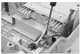
3.4 Install the cable onto the bracket, secure with hook and loop fastener and secure the aramid yarns if needed.
