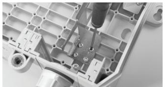
3.2 Install the cable bracket into the box..
