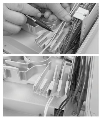
3.6 Route the loose tube towards the tube holder and strip.
