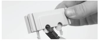
1.1 Different wrap-around ports are available (including brackets). Use two guiding pins to open the ports and to secure the bottom part to the box. Cut out the plastic part if you want to install a cable.
