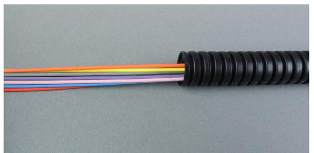
3.2 Feed the fiber through the flex tube
