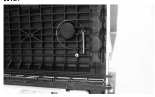
9.11 Hook the spring at the latch right end and then close the latch.
