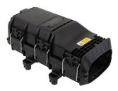
OFDC B8G Fiber Optic Splice/Patch Closure, Gel Cable sealing, 4 preinstalled 12 fiber trays , 1 pre-installed 18 fiber splice tray, 8 duplex LC /APC adapters, 16 pigtails, no splitter
