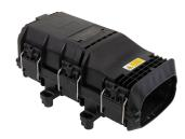
OFDC B8G Fiber Optic Splice/Patch Closure, Gel Cable sealing, 6 preinstalled 12 fiber trays , 8 duplex LC/APC adapters,  $2x\ 1-8$  splitter preconn at drop side
