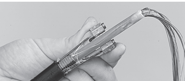
4.3.7 Install the strength member termination plate.
