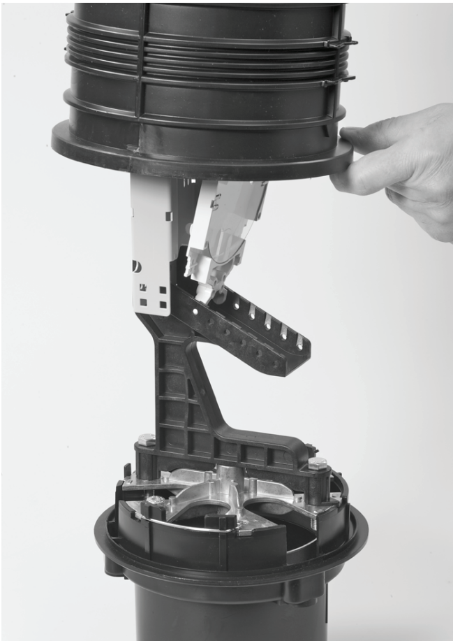
3.3 Fix the work stand to the table. Install the frame on the work stand. There are two positions to mount it on the work stand (FOSC-450-CAPH-B/D).
