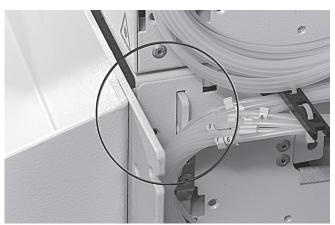
4.2.3 Insert the right side (back bracket) into the slot in the side panel of the shelf.
