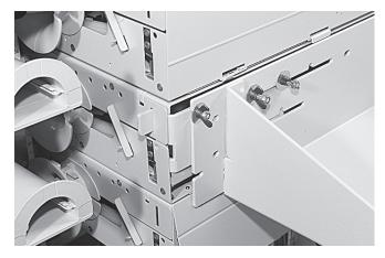
4.2.4 Loosen the wing nuts of the left bracket and adjust the bracket till it fits into the slot in the side panel of the shelf. Tighten the wing nuts properly.
