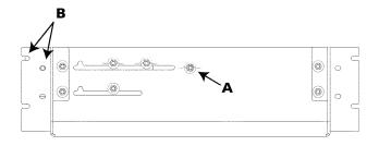
4.2.5 Remove the threaded rod with wing nut (A) and insert (screw) into the appropriate hole (ETSI or 19") (B).
