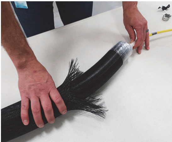
Figure 16. Removing the Pulling Sock
