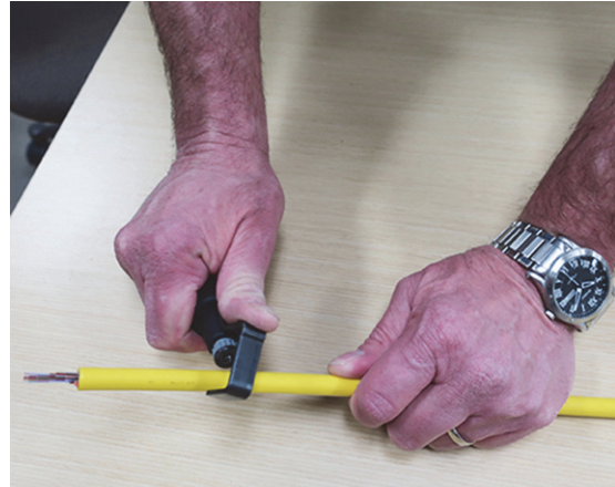
Figure 8. Stripping the Cable
