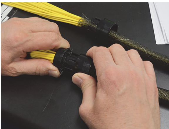
Figure 11. Installing the Cable Gland
