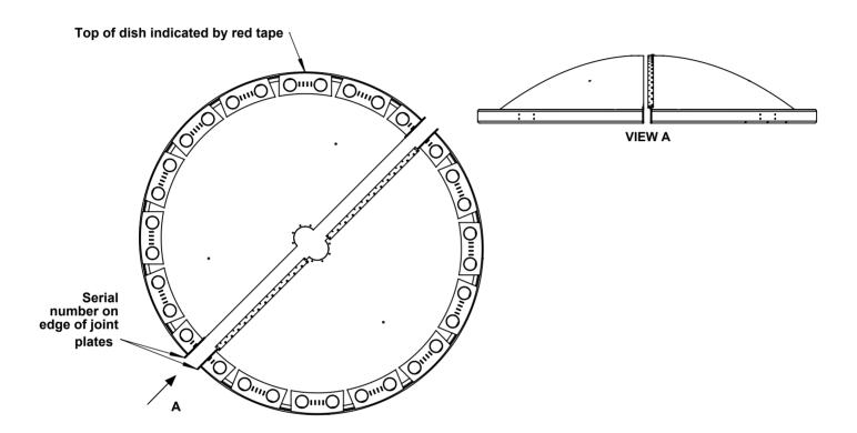
Install M8x30 bolts at locations as shown, 7 at each joint plate.
