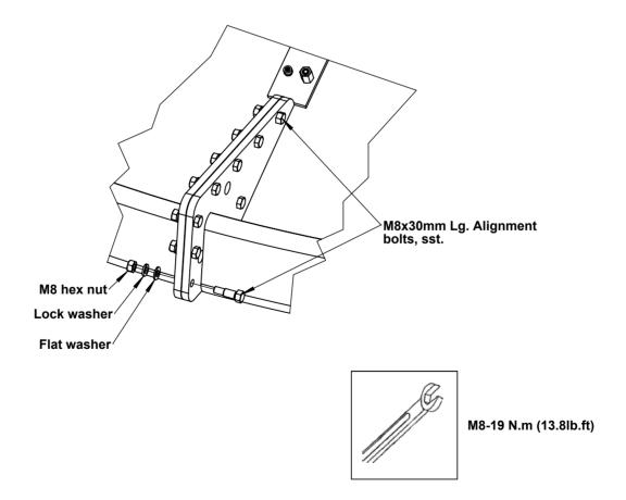
Add remaining splice strip bolts and tighten from rim to feed hole, one side at a time. The seam gap must be made uniform prior to tightening splice strip bolts. The seam gap can be opened by person under the reflector pushing outward at the seam, and closed by person outside dish pushing inward at seam.
