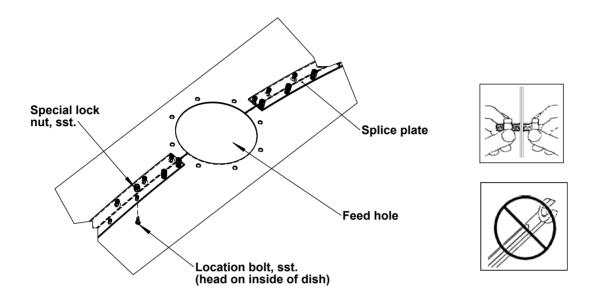
Install and tighten 4 alignment bolts at locations shown, 2 at each joint plate. bolts should insert easily by hand, remove paint from holes if necessary. Tighten all bolts at joint plate after alignment bolts tightened.
