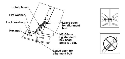
Install 6 location bolts and lock nut in splice plate, 3 on each side of feed hole
