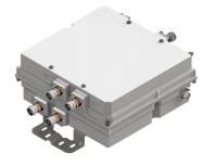
Dual Band Tower Mounted Amplifier, 700//900 MHz, 12 dB, 2 BTS & 4 ANT ports, AISG with 1 RET connector (1 device with 2 sub-units), with 4.3-10 connectors
