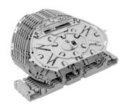
FIST® Splice Sub-assembly kit with 8 foldable dual circuit trays, each for holding up to 2x2 primary coated fibers, with Heat Shrink type splice holder
