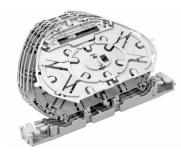
FIST® Splice Sub-assembly kit with 4 foldable dual circuit trays, each for holding up to 2x2 primary coated fibers, with Heat Shrink type splice holder
