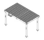
Equipment Platform, 8 ft x 14 ft, base with four 7ft x 6in OD Helicals
