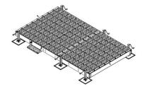
Equipment Platform, 8 ft x 14 ft, base with four adjustable feet
