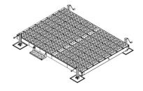
Equipment Platform, 8 ft x 11 ft, base with four adjustable feet
