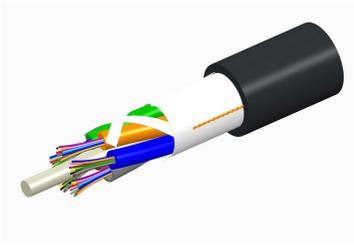
Fiber indoor/outdoor cable, LightScope® ZWP, Single Jacket All-Dielectric, Low Smoke Zero Halogen (LSZH), Singlemode G.652.D and G.657.A1, 24 fiber, Gel-Free, Stranded Loose Tube, Feet jacket marking, Black jacket color, Cca flame rating
