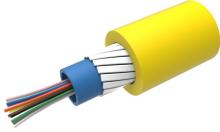
Fiber indoor/outdoor cable, LightScope® ZWP, gel-filled, loose tube, 24 fiber, yellow, Singlemode G.652.D and G.657.A1, Yellow jacket color, Dca flame rating. Provides Rodent Resistance
