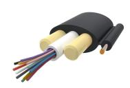
Tone Wire Outdoor Drop Cable, 12 fiber Arid Core construction, central loose tube
