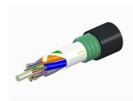
Fiber indoor/outdoor cable, TeraSPEED®, Single Jacket/Single Armor, Low Smoke Zero Halogen (LSZH), Singlemode G.652.D and G.657.A1, 144 fiber, Gel-Free, Stranded Loose Tube, Meters jacket marking, Black jacket color
